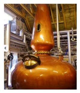
The proposed system will allow production of 16,650 litres of pure alcohol ("LPA") per annum - equating to 26,220 bulk litres of whisky. The Forsyths system will provide a full distilling process for the desired artisan, small batch quantities and also provide the stunning visuals which are vital to the visitor centre experience at the heart of the Barra Distillery project.
